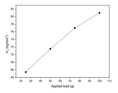
Fig.2: Load dependence of hardness for diglycine lithium sulfate crystal
