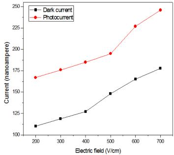
Fig.3: Variations of photocurrent and dark current with the applied field for Diglycine Lithium Sulfate crystal
