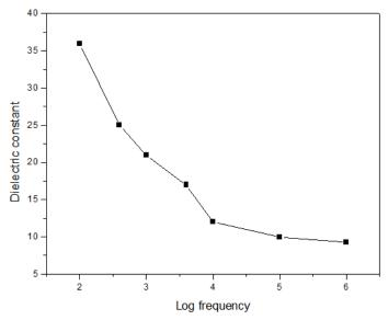
Fig.4: Variation of dielectric constant with frequency for Diglycine Lithium Sulfate crystal at room temperature
