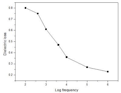
Fig.5: Variation of dielectric loss with frequency for Diglycine Lithium Sulfate crystal at room temperature
